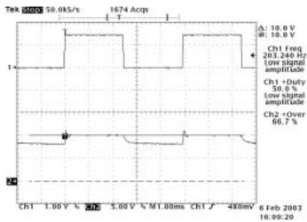
Channel 1 is the Enable waveform Channel 2 Output Voltage reacting to Enable signal
